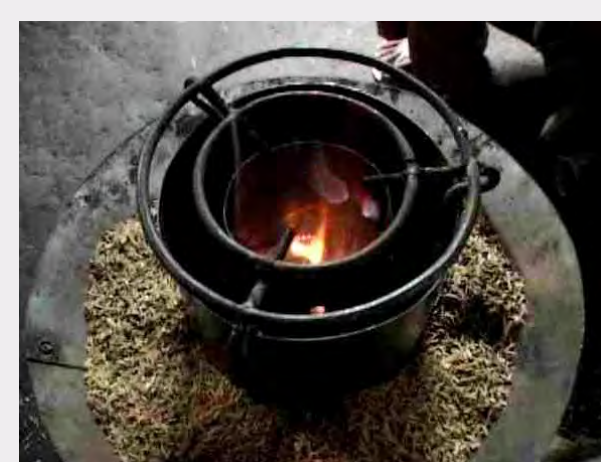
Non-fan assisted clean combustion blue flame of the Mayon Turbo Stove
